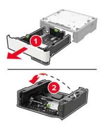
**5** Remove the used pick roller assembly.
