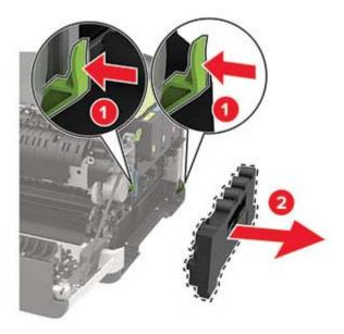
Note: To avoid spilling the toner, place the bottle in an upright position.
