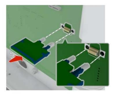
**Note:** The entire length of the connector on the card must touch and be flush against the controller board.
