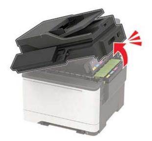
**CAUTION—HOT SURFACE:** The inside of the printer might be hot. To reduce the risk of injury from a hot component, allow the surface to cool before touching it.
