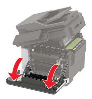
3 Open the fuser access door, and then remove the jammed paper.Note: Make sure that all paper fragments are removed.
